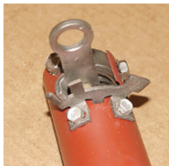
Photo #1: The original automatic steering column utilizes a bolt-on shifter detent at the bottom of the column available as P/N 19-38 or 19-39 . This detent positively locks the column shift arm in the "Park" position, keeping the transmission safely locked into "Park".
