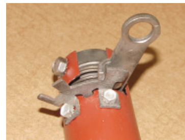
Photo #2: The original shifter detent will only allow the shift arm to travel far enough to operate a Powerglide or Turboglide transmission.
