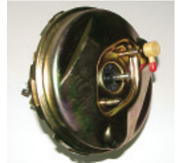
Photo #2: Not all 1968 to 72 A and F-body cars had the shallow dimple style master cylinder. Some applications used the master cylinder with the deep hole in the piston and required a booster with a long master cylinder pushrod.
