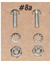
Photo #8a, 8b & 8c: The new adjuster brackets are attached to the bucket with two #10-32 X 3/4" machine screws, serrated washers and nuts supplied with the kit.
