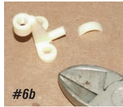
Photo #6a & 6b: The replacement adjuster brackets included in kit P/N 34-100 are made of nylon and attach to the headlight bucket using the supplied hardware. There is a tail on the replacement bracket that must be removed for this application. Using a pair of side cutters, remove half of the tail.
