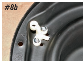
Photo #8a, 8b & 8c: The new adjuster brackets are attached to the bucket with two #10-32 X 3/4" machine screws, serrated washers and nuts supplied with the kit.
