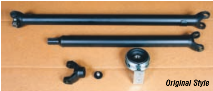
Photo #1: Shows the complete original style drive shaft system. The short shaft with the splines is the front half of the driveline.
